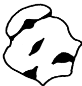
Fig. 8.1 Illustration of a porous fragment and bulk, apparent, and ultimate density values.
