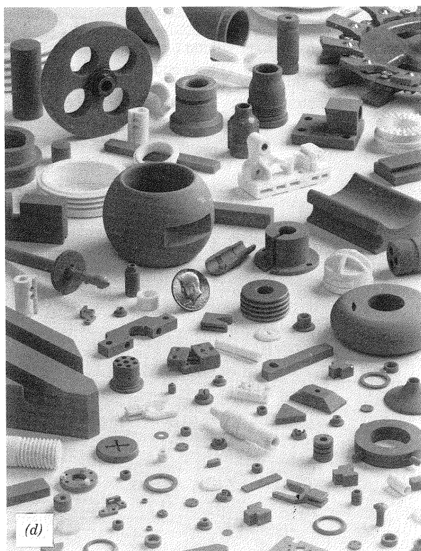
Fig. 1.1(d) Advanced alumina structural ceramics used in a wide variety of materials-processing technology applications (textile guides, valve seals, impellers, nozzle inserts, wear blocks, cutting tools, milling media, refractory insulation supports) and electrical applications (spark plug insulators, electronic substrates, electrical insulation). (Photo courtesy of Diamonite Products Div., Ferro Corporation, Shreve, OH.)
